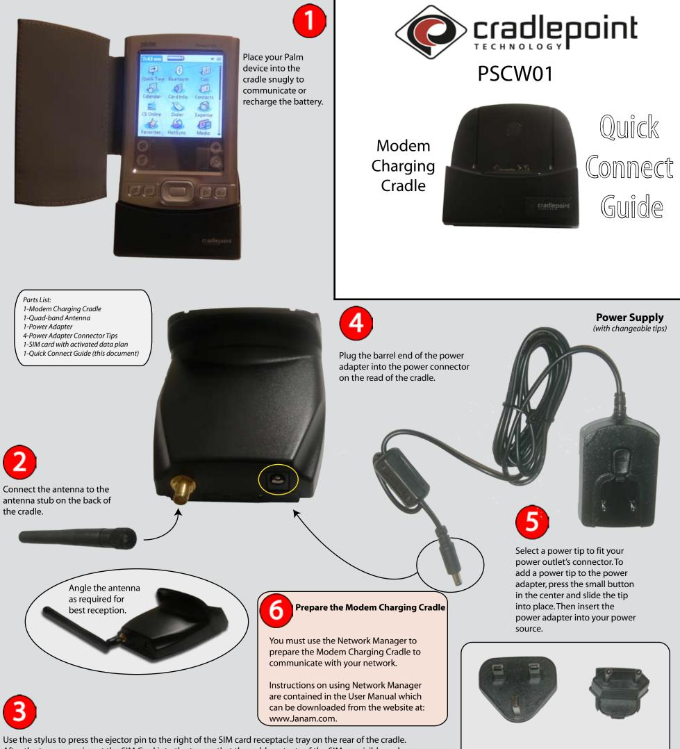
Use the stylus to press the ejector pin to the right of the SIM card receptacle tray on the rear of the cradle. After the tray opens, insert the SIM Card into the tray so that the gold contacts of the SIM are visible and the notched corner of the card matches the notched corner of the tray and then press the receptacle back into the cradle.
